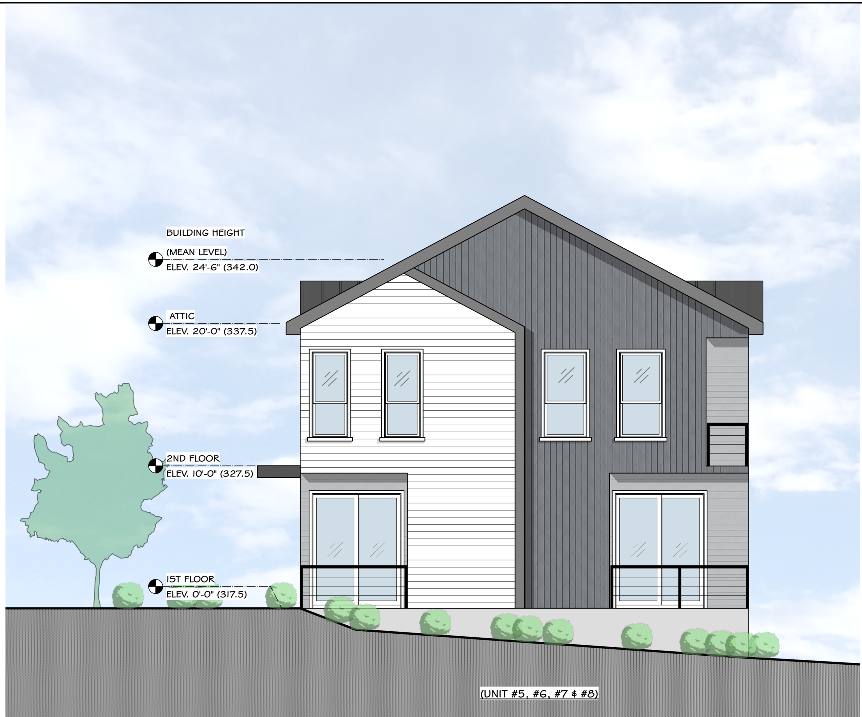
2 PROPOSED BUILDING ELEVATION (TYP.) Scale: 1/4" = 1'-0"
